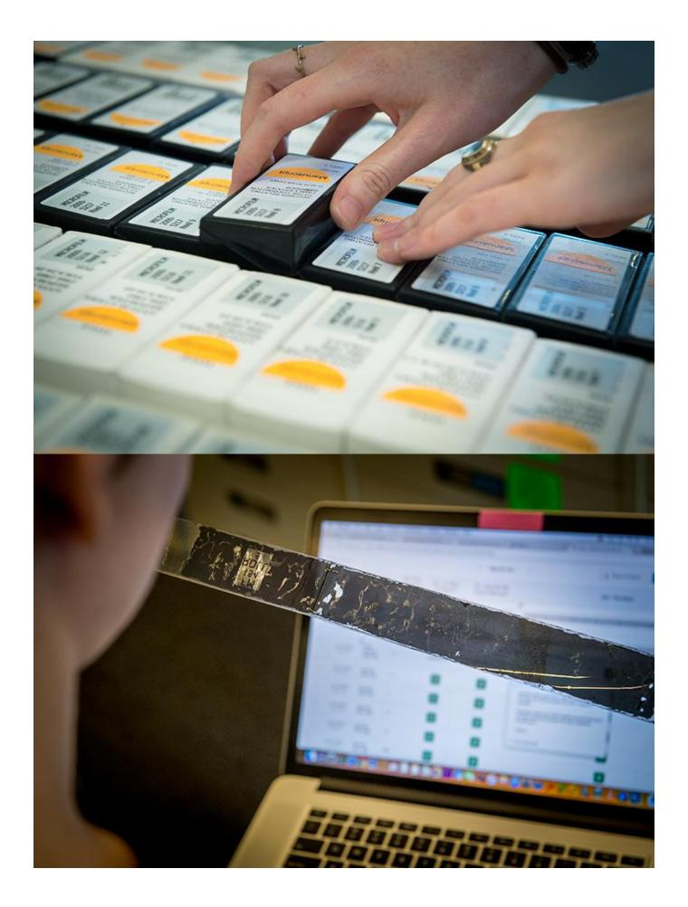
A-D strips are designed to be used for testing acetate film in any format: sheet film, roll film, cinema film, or microfilm. Originally blue, the strip changes color according to the severity of the level of acidity. The more yellow the color, the higher the level of acidity.
