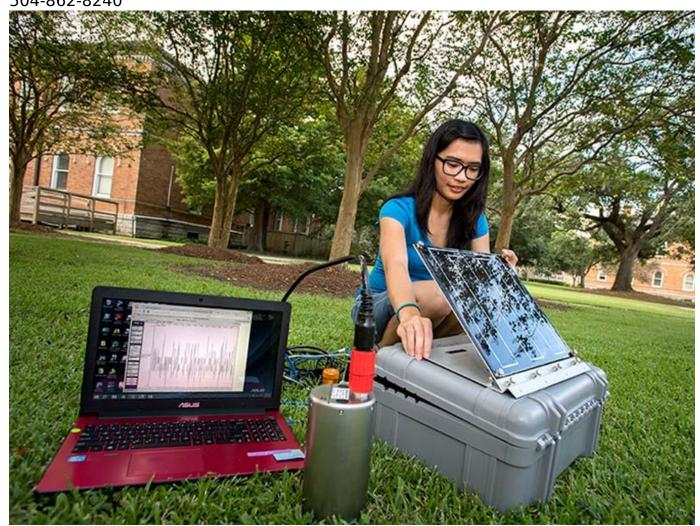
Sarah Oliva, a PhD student in earth and environmental sciences tests a seismometer in the quad near Blessey Hall. The state of the art equipment is headed for New Zealand where it will monitor unusual volcanic earthquakes. The data will help researchers understand the inner workings of a volcano. (photo by Paula Burch-Celentano)
