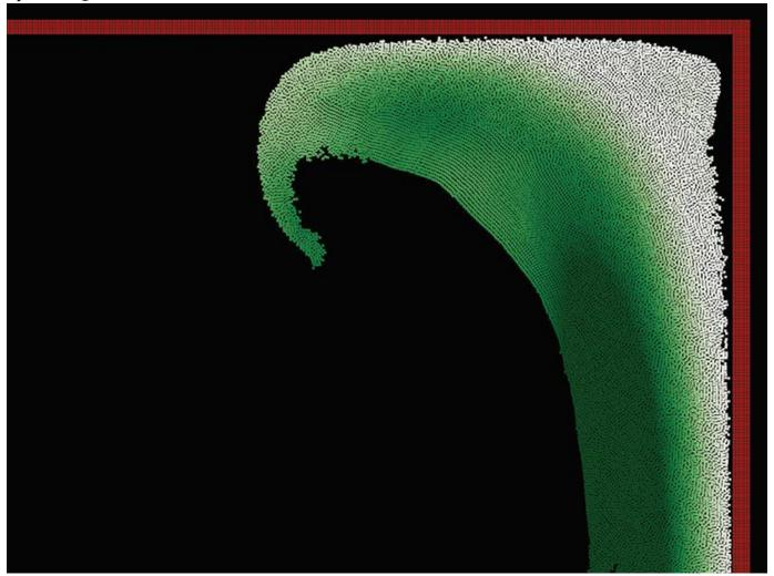
This image depicts a dam-break wave at a vertical wall as computed using the moving particle semi-implicit method. It was on display at the Center for Computational Science art show in fall 2016.
