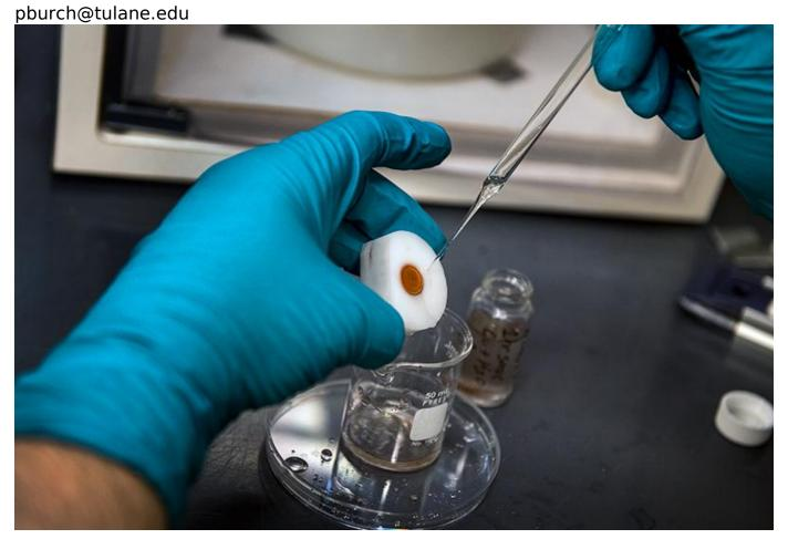
After creating eroded copper particles, Jeremy Wright, a doctoral candidate working in the lab of professor Brian Mitchell in the Tulane Department of Chemical and Biomolecular Engineering, transfers the particles for analysis to determine if nanoparticles are present. The nanoparticles will eventually be used to create metal-based 3D printed objects with finer features.
