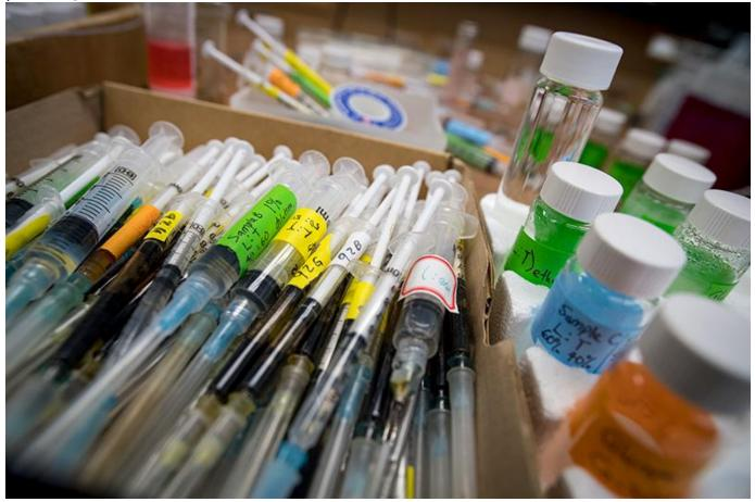
In the lab of Kyriakos Papadopoulos, in the <u>Department of Chemical and</u> <u>Biomolecular Engineering</u>, researchers experiment with various crude oil samples and chemicals (pictured) in search of ways to treat crude oil-contaminated sand using an environmentally safe approach.
