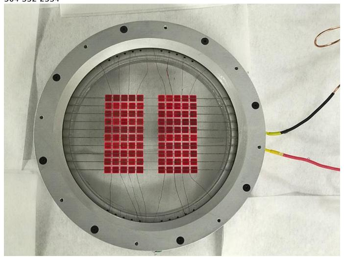
The hybrid solar energy converter features a solar module with glowing red cells built at Tulane. (Photo courtesy of Matthew Escarra)
