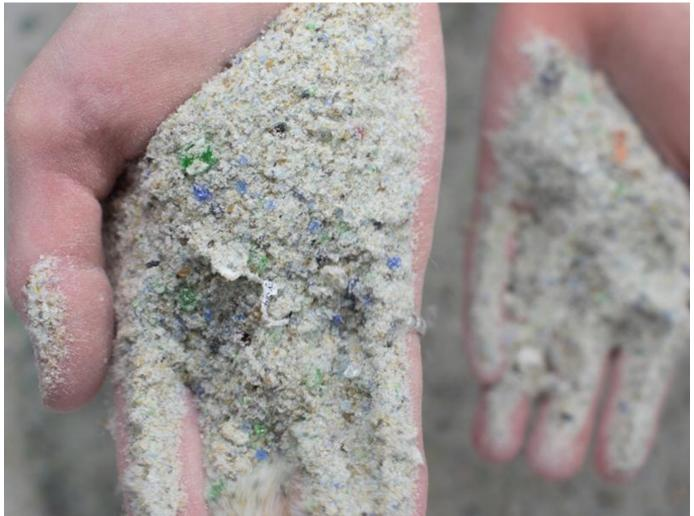
Glass Half Full NOLA collects and converts glass bottles into sand and glass cullet, which can be used for coastal restoration, flood prevention, eco-construction and new glass. (Photo courtesy of Max Steitz)
