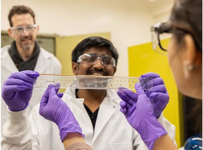
Bullet-proof superhero-style suits seem like the stuff of fiction, but a team of researchers at Tulane University is working to develop a material that could make them a reality. Here, they are measuring how much a piece of the material they produced can stretch. (Photo by Kenny Lass)
