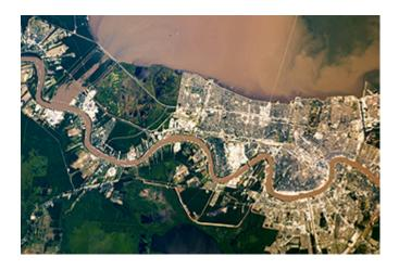
The Bonnet Carre spillway (shown in the upper left) is located along the Mississippi River 12 miles upriver from New Orleans. This river control structure and the Morganza spillway, 35 miles upriver from Baton Rouge, were opened this spring to alleviate the threat of flooding in urban areas. (Satellite photo from NASA)
