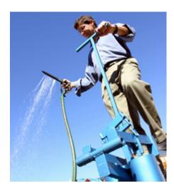
Kickstart founder Martin Fisher demonstrates how to use a pedal-powered water pump that allows farmers to push water uphill and improve their crop production. (Photo courtesy of Lemelson-MIT Program.)
